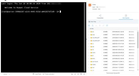
Figure 8-9 Viewing the file list of a Linux host
